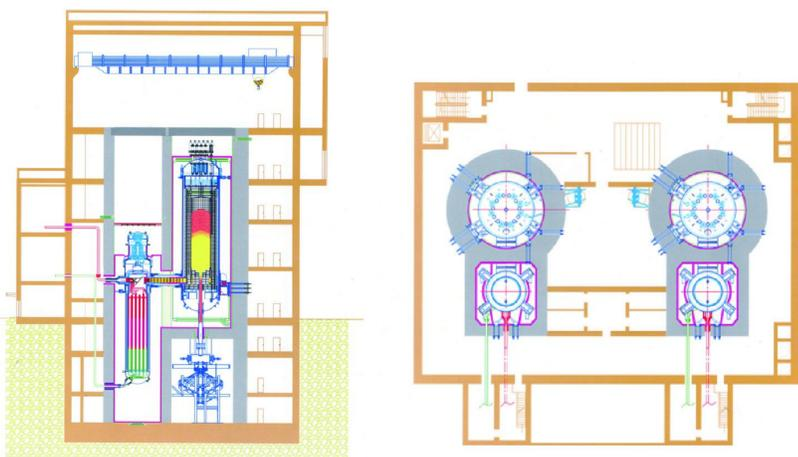
Figure 1. The layout of the HTR-PM demonstration plant in Huaneng Shidao Bay site. A proposal for a 2x600 MWe unit consisting of six such twin-reactor modules passed initial feasibility review in 2015 for a site in Ruijin City, People's Republic of China.
