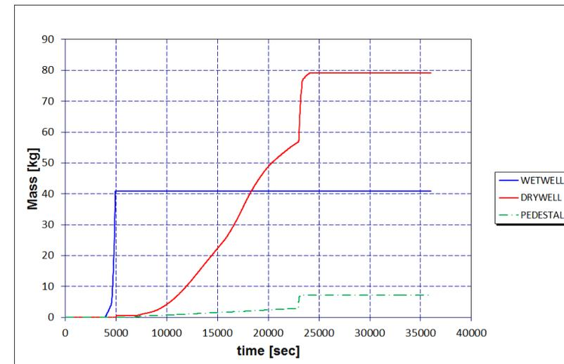
*Mass of burned  $H_2$  in non-inerted containment.*
