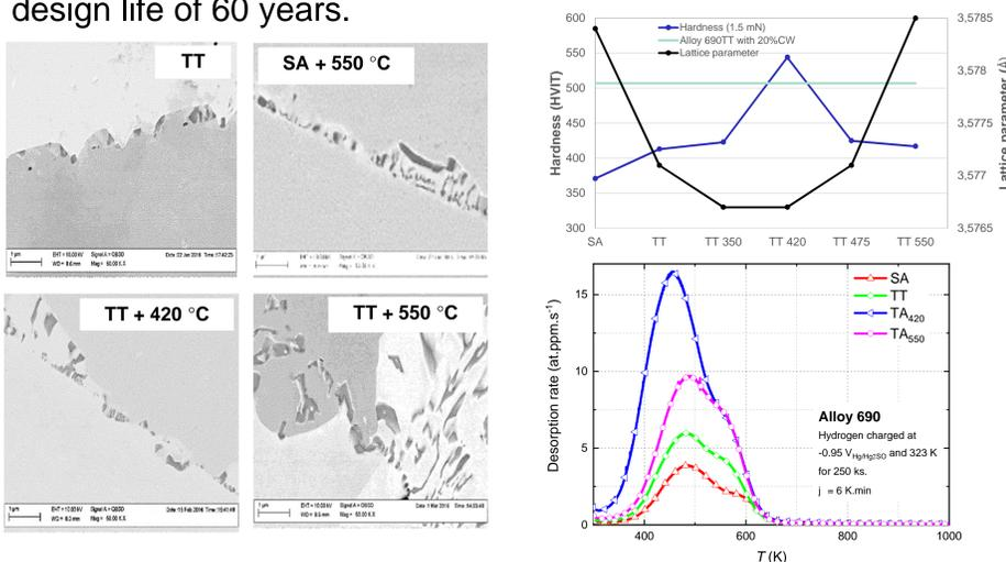
**Figure 1.** Thermal ageing of Alloy 690 causes IG carbide growth (left) and lattice contraction (upper right), which indicates SRO. Thermal ageing of Alloy 690 increases hydrogen uptake during charging (lower left).
