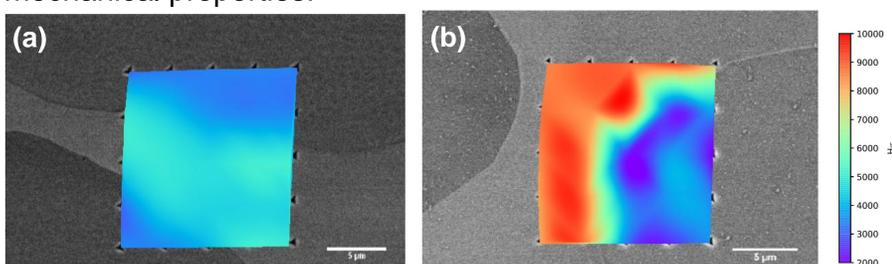
**Figure 2.** Thermal ageing increase the nano-hardness of the ferrite phase in the dual phased cast stainless steel. In (a) the solution annealed condition and (b) thermally aged condition of the hot leg material are shown.
