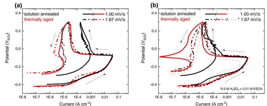
**Figure 3.** The electrochemical response is stronger with slower scan rate in both the (a) hot leg and (b) cold leg materials. The response vs thermal ageing is not straightforward, as it is for laboratory aged materials.
