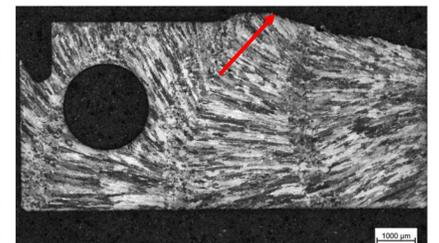
**Figure 4.** Typical microstructure of RPV weld metal. The arrow shows the location of brittle fracture initiation.
