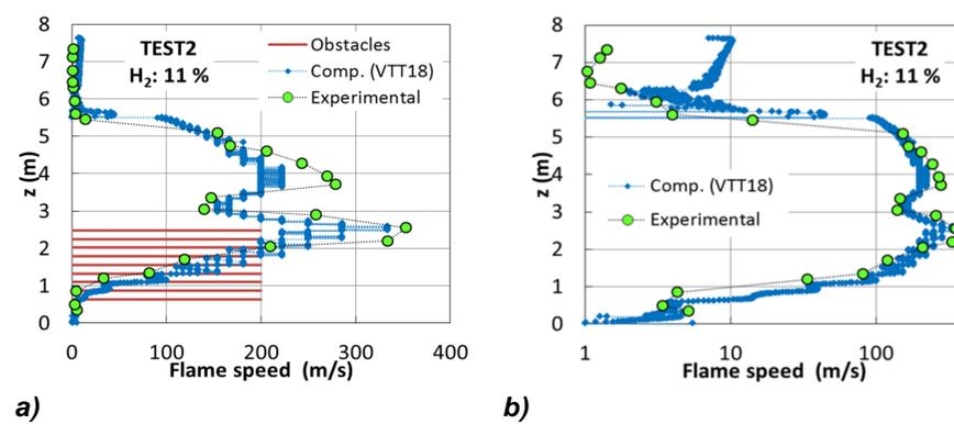
**Figure 3.** Computed and experimental flame speed in Test 2 of the Etson-Mithygene benchmark a) with and b) without obstacles that accelerate the flame propagation as in real containment rooms.
