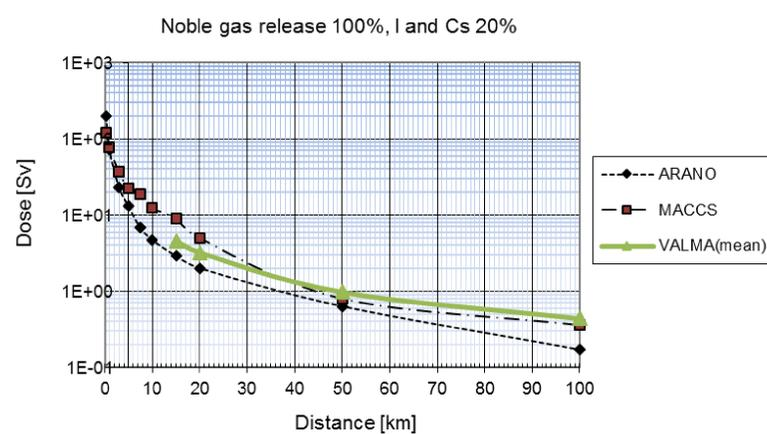
**Figure 4.** The dose of 95% fractile as a function of distance from the power plant. Integration time is one year for external radiation from the ground.
