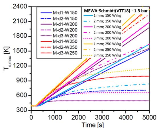
**Figure 2.** Comparison of the time evolution of the maximum solid particle temperature for the truncated-cone debris beds in the MEWA simulations of this study and in the DECOSIM simulations by Yakush & Kudinov, 2014. In the MEWA simulations, the top surface pressure is 1.3 bar.
