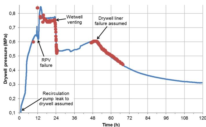
**Figure 1.** Fukushima unit 1 pressure in the containment drywell during the accident. Red dots are measured values and blue curve is the result from the MELCOR simulation.
