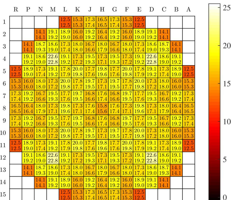
**Figure 1.** Radial power distribution in the hot full-power state of a PWR core (MIT BEAVRS benchmark). The values are assembly powers in MW calculated using a reference Serpent 3D model (top) and the Serpent-ARES code sequence (bottom).
