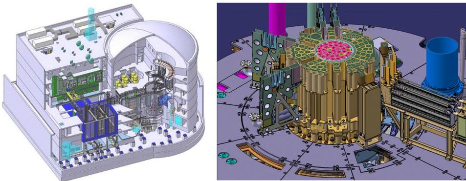
**Figure 1.** Left figure: The layout of the Jules Horowitz Reactor complex, with reactor building located in the right, spent experimental fuel storage pools in lower left side and the hot cells for specimen preparation and examination upper left.
