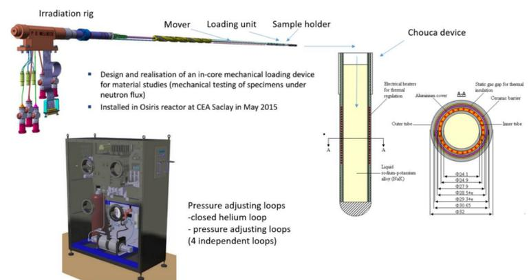
**Figure 2.** The MeLoDIE experimental setup includes a sample holder, a Chouca irradiation capsule, a glove box containing a gas management system and a safety box for the sample holder, another glove box for the Chouca capsule, above-water lines and underwater lines for connecting the pneumatic and electrical lines between the glove box and the sample holder.
