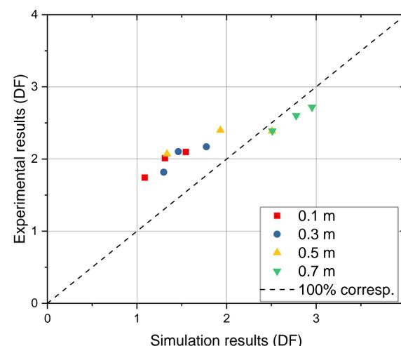
**Figure 3.** Comparison of experimental and simulated (ASTEC) decontamination factor (DF) results. Experiments were performed with Csl aerosol at 20 °C varying the pool depth from 0.1 to 0.7 m and non-condensable N<sub>2</sub> flow rate through the pool from 8, 14 to 27 l/min.
