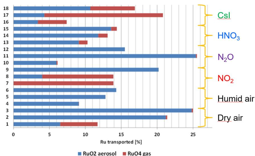
**Figure 1.** Transport of ruthenium as gaseous and aerosol compounds. Air radiolysis products may significantly increase the transport of (low volatile) ruthenium as a gaseous compound into the containment building (air ingress conditions). The highest transport of ruthenium as a gaseous compound was observed when Csl reacted with ruthenium oxides.
